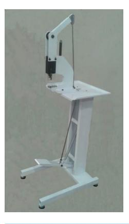
Pedal: version with mecanical's action with toggle, economic version, very versatile which allows the utilisation of dies called dies "C", as spherical punches and hollow punches, dies for eyelets, rivets, pression's buttons in all the forms and dimensions.
