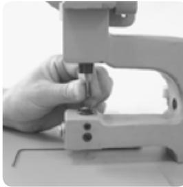
10. Now carefully insert the corresponding pilot pin into the cylinder. Make sure that it is in the proper place.
