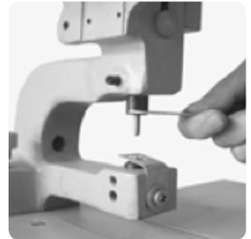
5. Unscrew the upper punch from the cylinder using the spanner.
