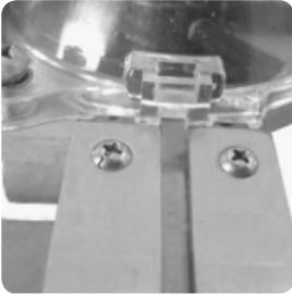
13. Now re-attach the magazine cover with both screws. Make sure that the lower magazine opening is positioned exactly above the eye channel.
