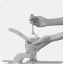
1. Remove the eyelets from the magazine.
