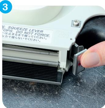
3 Unlock the bottom cover by sliding back the tab with the „open“ sign, and open the bottom cover.
