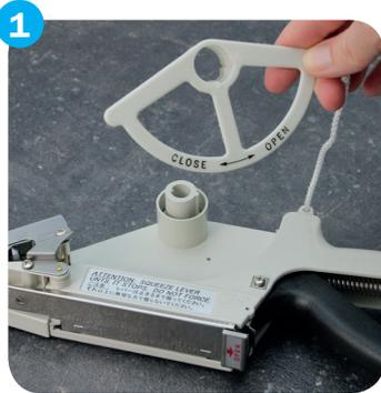
1 Twist the roll holder in a counterclockwise direction and remove it.
