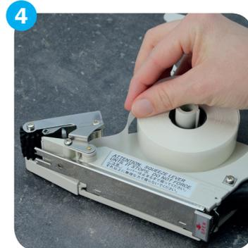
4 Guide the tape under the clear plastic plate. Turn back the tape via the nose section.
